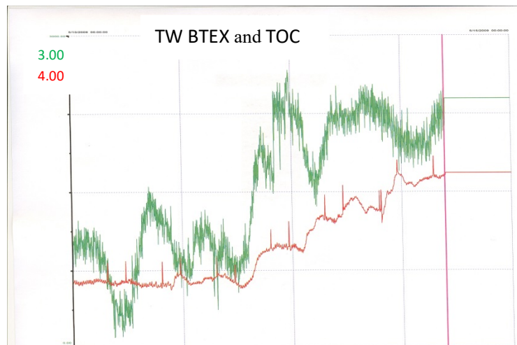
Figure 3: Boiler Feed Water measured by Total Organic Carbon Analyzer (Green) and Fluorescence Monitor (Red).
